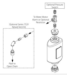
The retard chamber must be installed as shown on the alarm check trim drawings.
